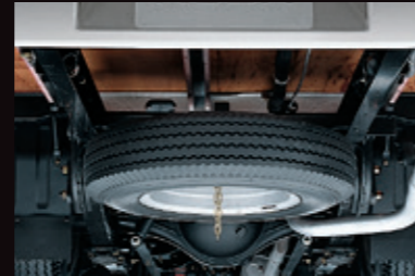
Spare tire under rear end
