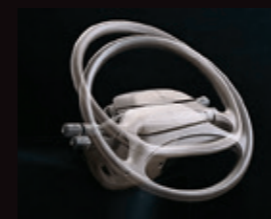
Protecting the driver Impact absorbing steering system
