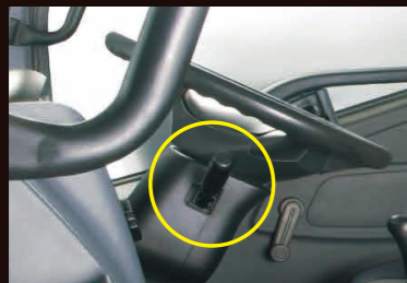
Exhaust brake located on the combination switch
